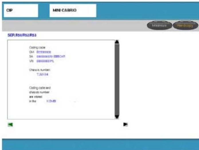
Fig. 15: Display Screen - ZCS Information For Vehicle Is Displayed Along With Stored Location Courtesy of BMW OF NORTH AMERICA, INC.
